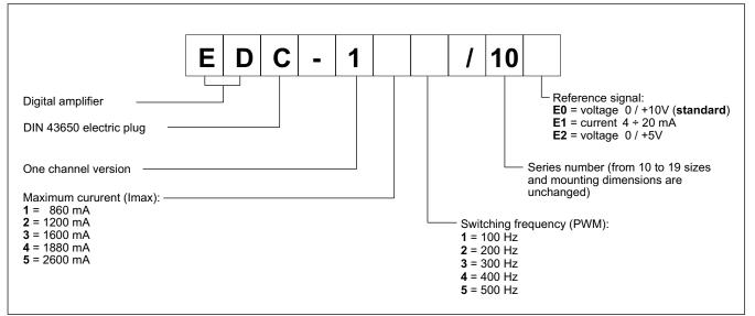
The EDC-1 connector is a digital amplifier controlling open loop proportional valves. The unit supplies a variable current in proportion to the reference signal and independently of temperature variations or load impedence.
